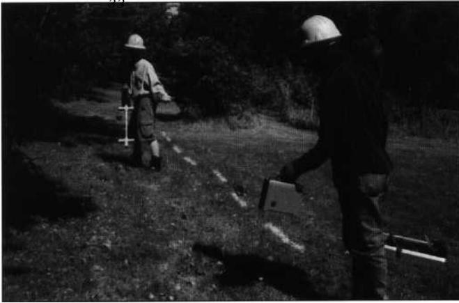
Using locating equipment in the inductive mode allows a team to verify a locate or to find unmarked lines.
